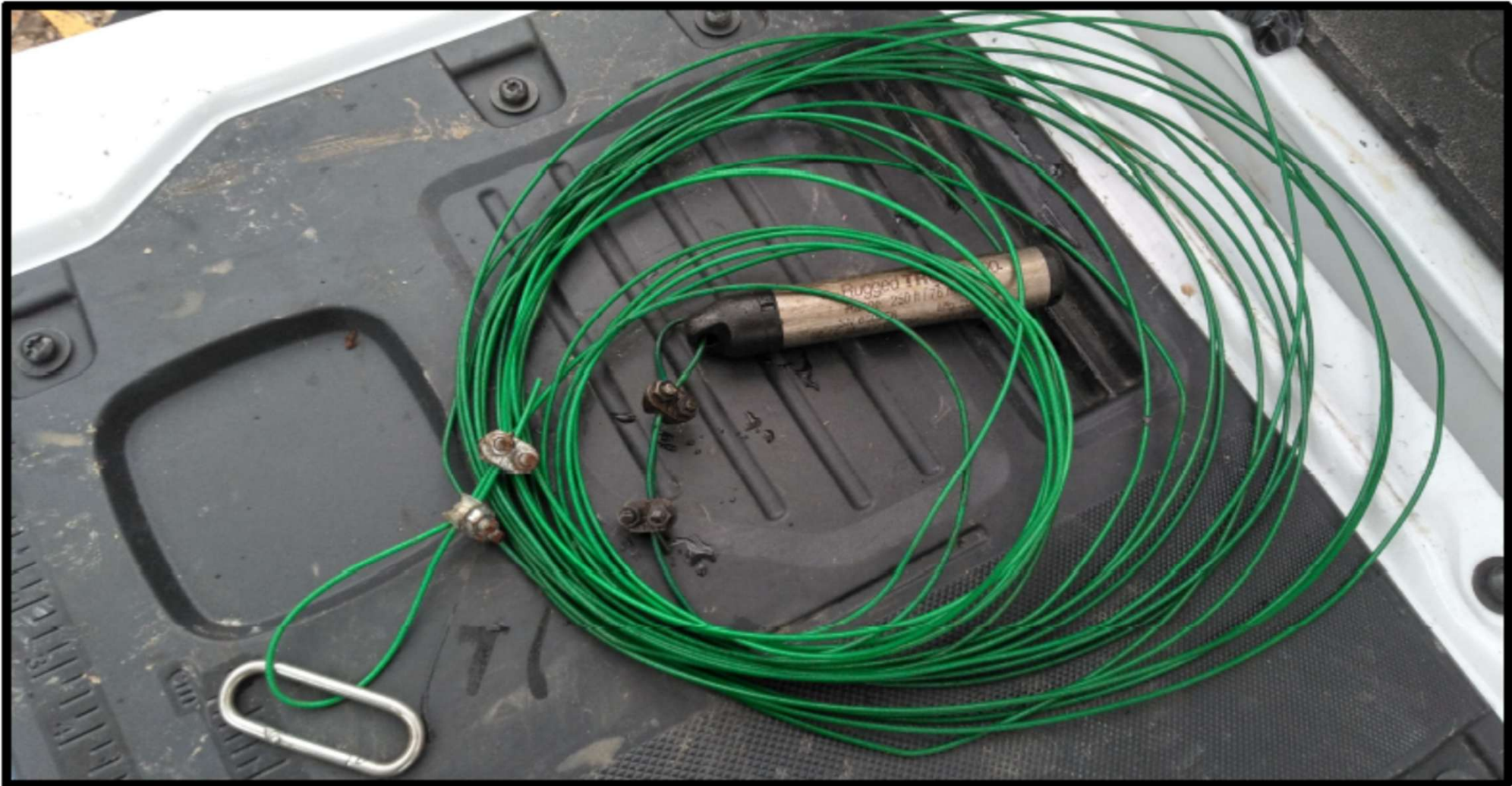
Hanging Wire Installation with Rugged Troll Transducer
